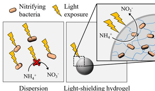
Fig. 1 Dispersed nitrifying bacteria and Light-shielding hydrogel under light irradiation.
