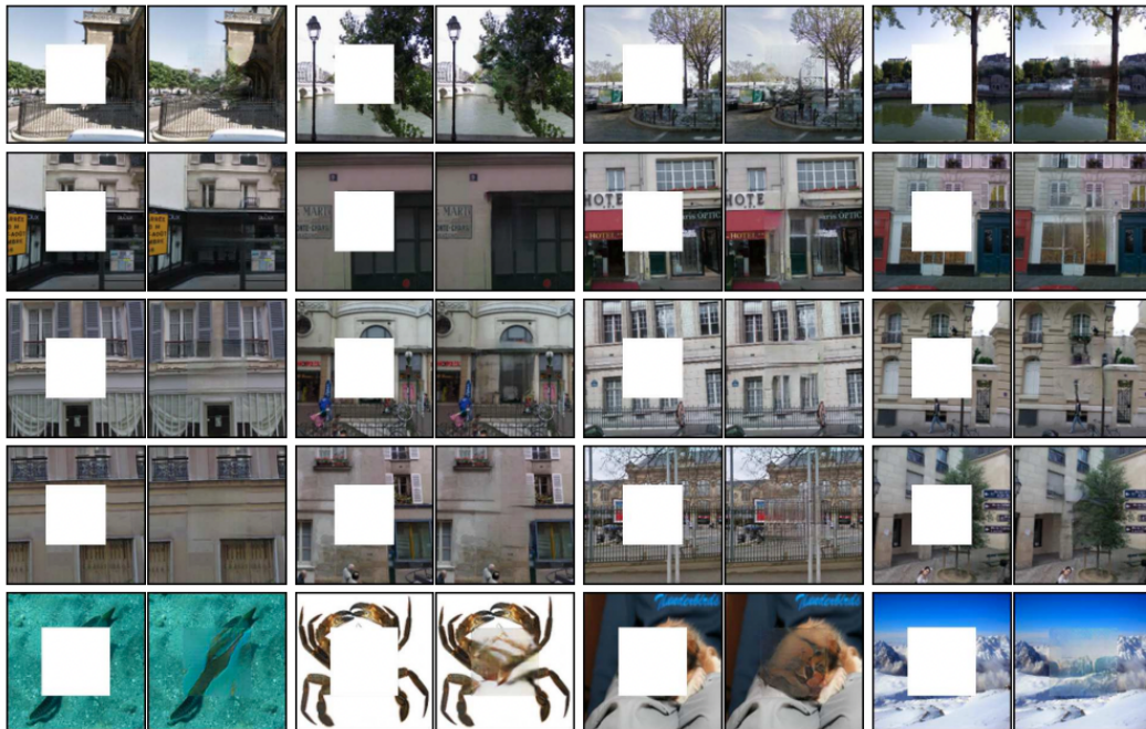
Figure 2.12: Semantic Inpainting results for context encoder trained jointly using reconstruction and adversarial loss. First four rows contain examples from Paris StreetView Dataset, and bottom row contains examples from ImageNet. Figure by Pathak et al. [265].
