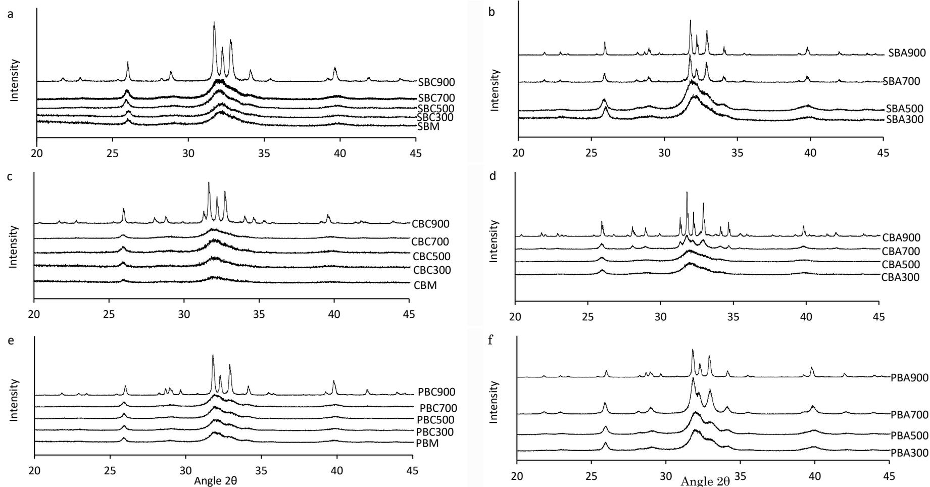
Figure 2-4. X-ray powder diffraction spectra from (a) sheep bone char (SBC) (b) sheep bone ash (SBA) (c) chicken bone char (CBC), (d) chicken bone ash (CBA), (e) pig bone char (PBC), and (f) pig bone ash (PBA) produced at 300°C (300), 500°C (500), 700°C (700), and 900°C (900). BM represents bone meal
