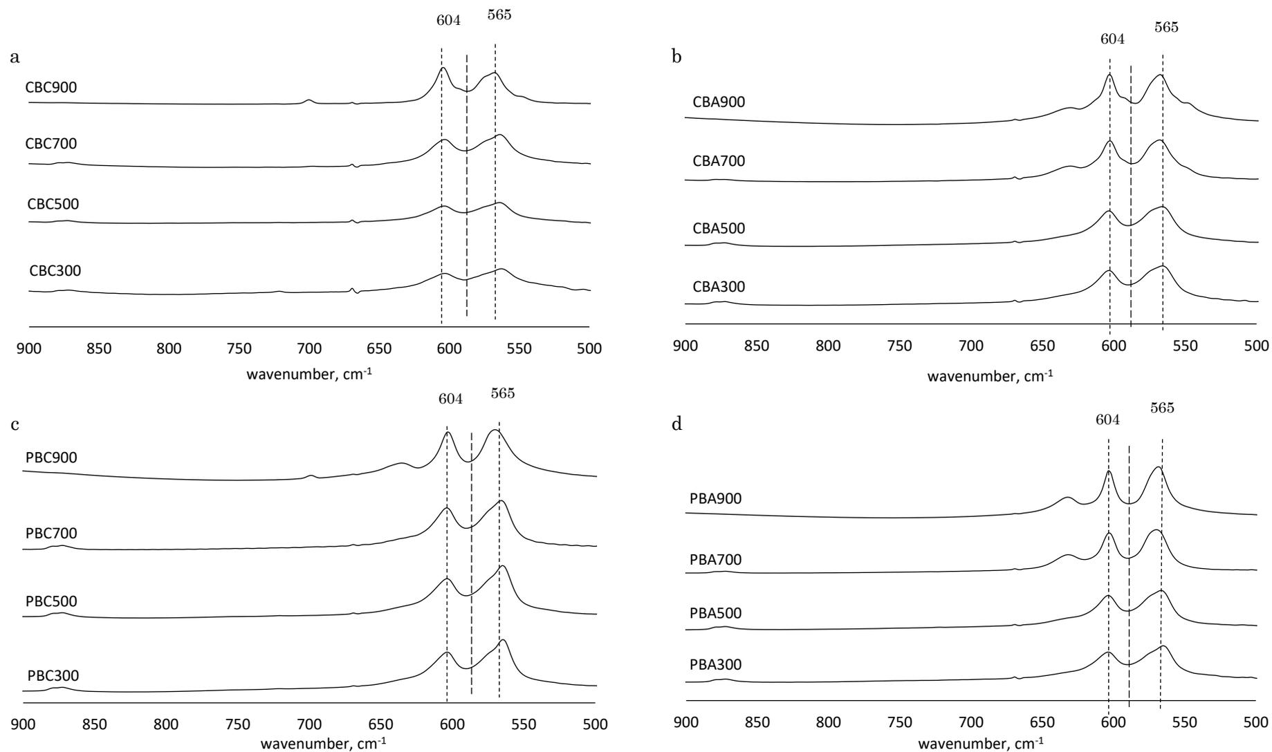
Figure 2-5. FTIR spectra ( $500 - 900 \text{ cm}^{-1}$ ) from (a) chicken bone char (CBC), (b) chicken bone ash (CBA), (c) pig bone char (PBC), and (d) pig bone ash (PBA) treated at  $300^\circ\text{C}$  (300),  $500^\circ\text{C}$  (500),  $700^\circ\text{C}$  (700), and  $900^\circ\text{C}$  (900). BM represents bone meal
