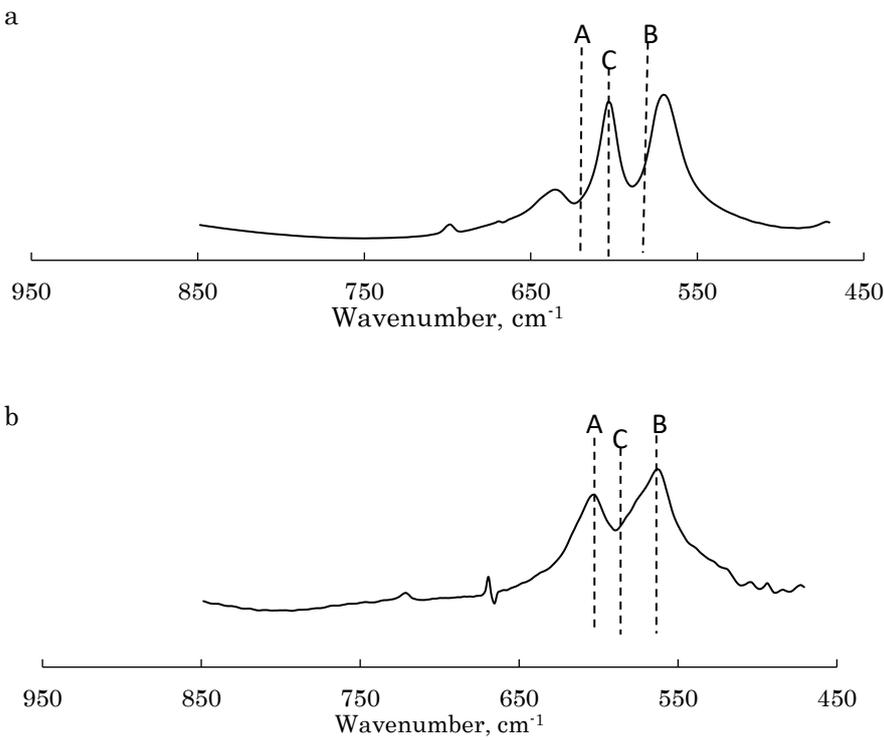
Figure 2-1. FTIR spectra of (a) pig-bone char produced at 900°C and (b) chicken-bone char produced at 300°C.
