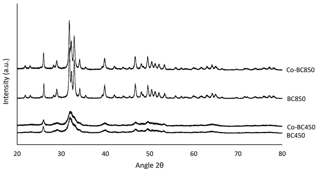
Figure 3-1. X-ray powder diffraction spectra from different bone chars produced at 450°C and 850°C
