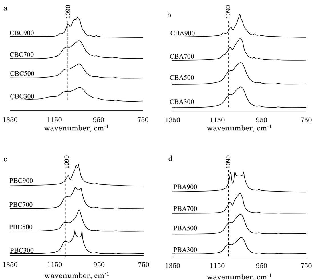
Figure 2-6. FTIR spectra ( $750 - 1350 \text{ cm}^{-1}$ ) of (a) chicken-bone char (CBC), (b) chicken-bone ash (CBA), (c) pig-bone char (PBC), and (d) pig-bone ash (PBA) produced at  $300^\circ\text{C}$  (300),  $500^\circ\text{C}$  (500),  $700^\circ\text{C}$  (700), and  $900^\circ\text{C}$  (900), respectively.
