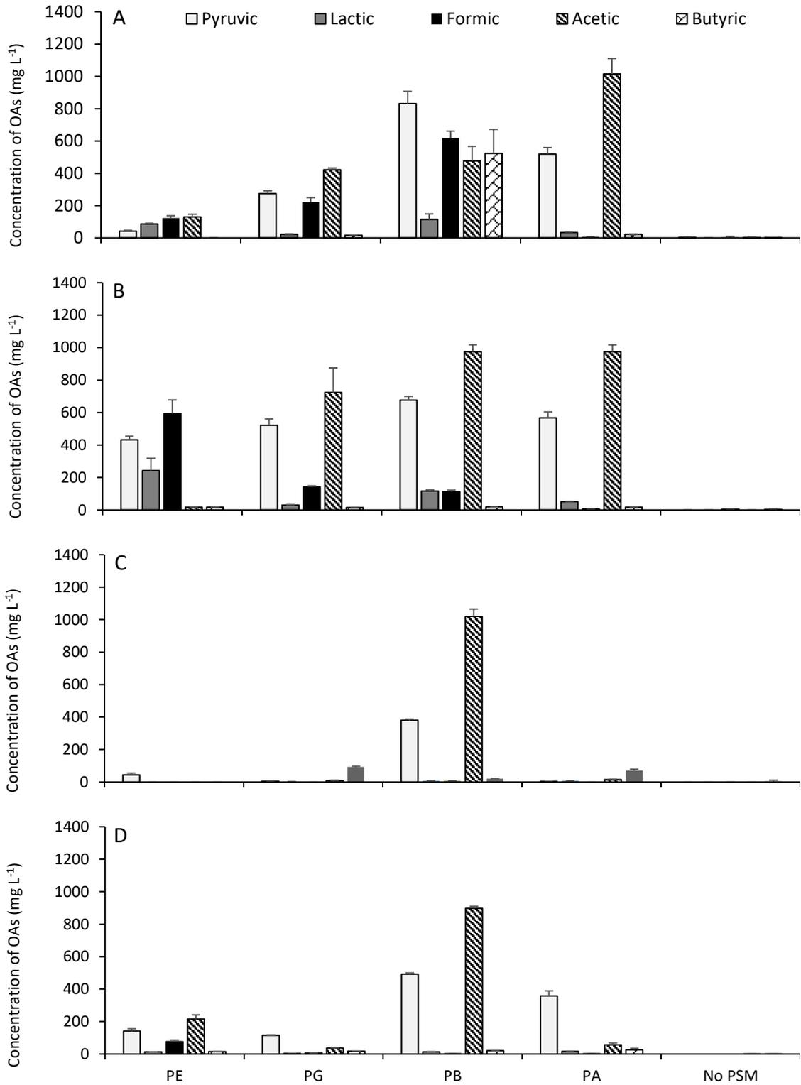
Figure 3-4. Concentration of carboxylic groups of low molecular weight organic acids produced by the strains at the different bone char types (A) BC450, (B) Co-BC450 (C) BC850, (D) Co-BC850 (only Day 14 data are presented)
