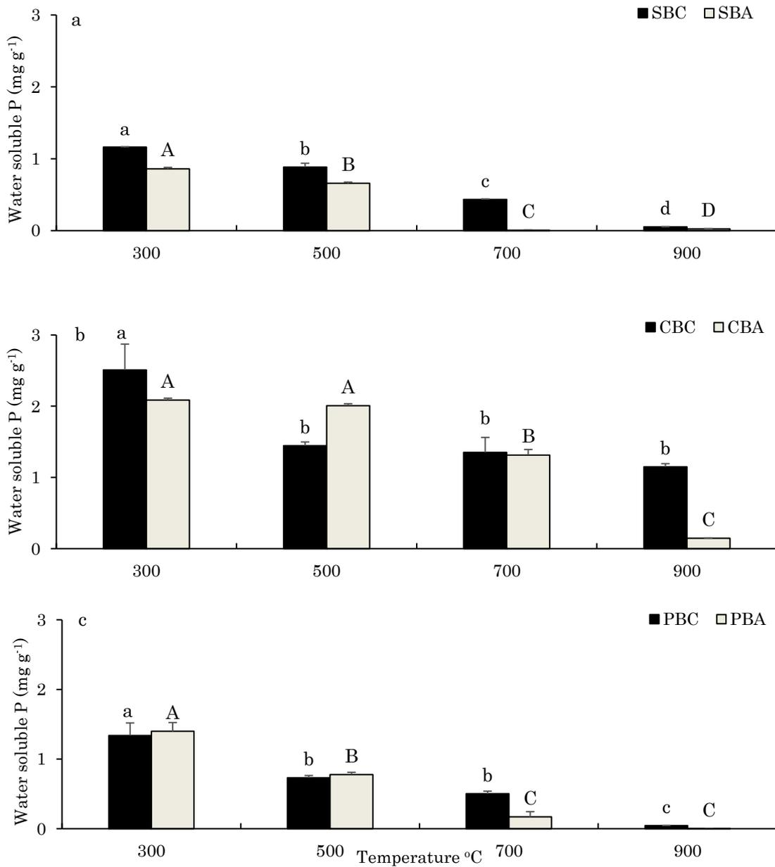
Figure 2-3. Water-soluble phosphorus (P) from (a) sheep bone char (SBC) and ash (SBA), (b) chicken bone char (CBC) and ash (CBA), and (c) pig bone char (PBC) and ash (PBA) treated at 300°C, 500°C, 700°C, and 900°C. Vertical bars represent standard errors ( $n = 3$ ). Same letters indicate no significant differences ( $p < 0.05$ ) in water P among different temperatures for different animal bone char (small letter) and bone ash (capital letter), respectively.
