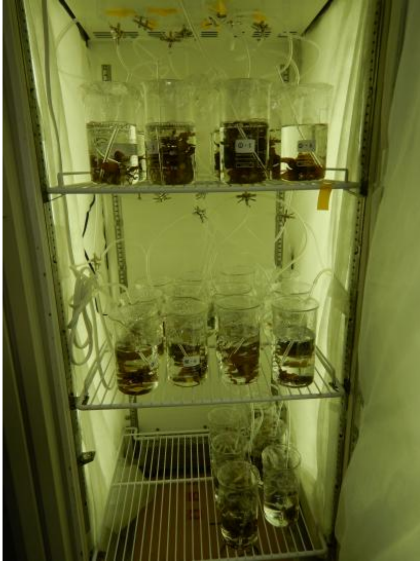
Figure 3-2 The incubator (MLR-350HT) used in study 2. The 600 mL-glass beakers with a total volume of 500 mL of seawater enriched with \text{NaNO}_3 , \text{NH}_4\text{Cl} and \text{NaH}_2\text{PO}_4 were set in the incubator. In all beakers, the culture media were gently supplied with air pumped through sterile silicon tubes.
