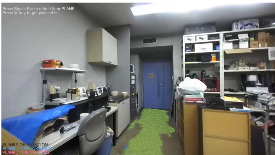
FIGURE 3.14: The ground plane extracted and overlay on the RGB image at step 2. The yellow mesh shows the safe area for the VIP to walk on
