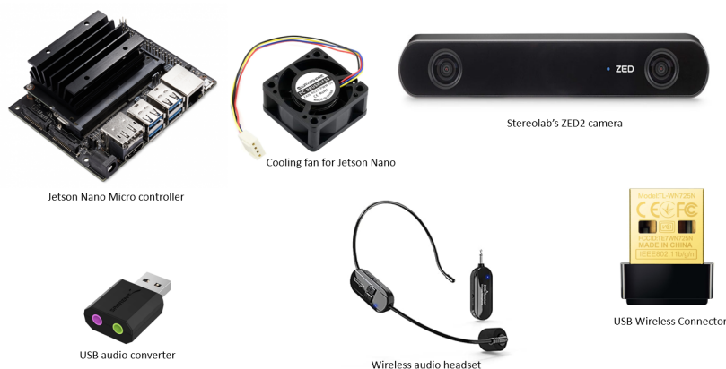
FIGURE 3.7: Various electronic components that were connected to design the wearable assistive device.
