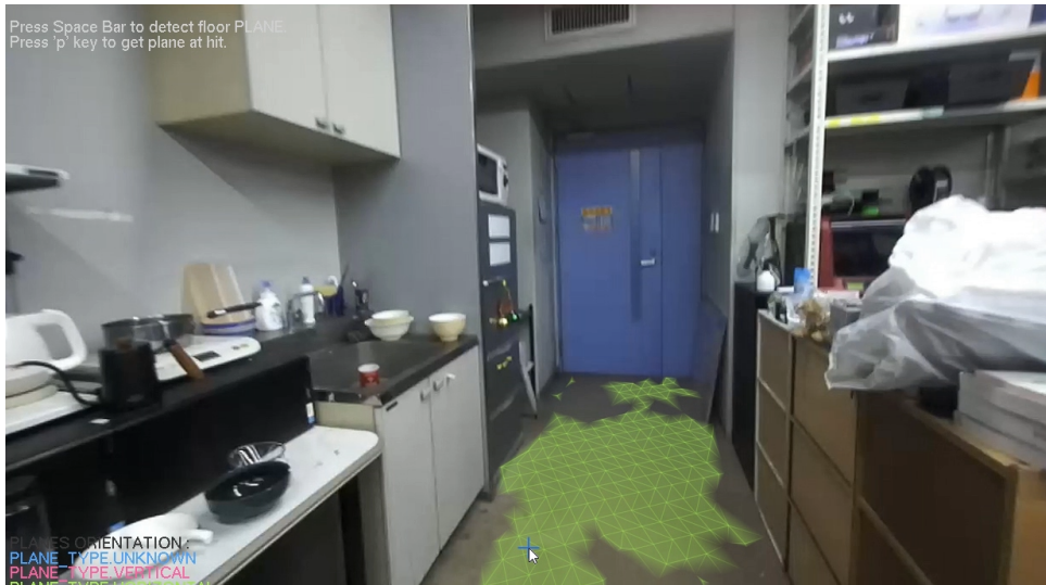
FIGURE 3.13: The ground plane extracted and overlay on the RGB image at step 1. The yellow mesh shows the safe area for the VIP to walk on
