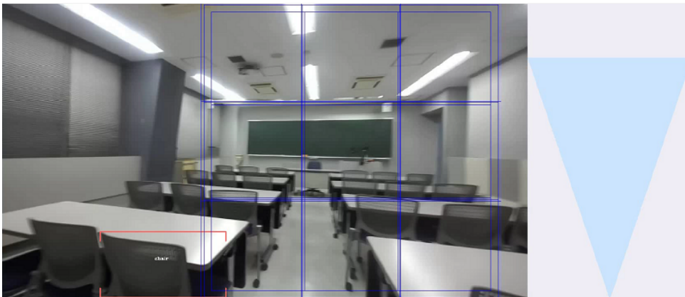
FIGURE 3.10: A screenshot showing the multiple adaptable grid boxes indicated with blue lines created for each detected object and used in determining the object in the proximity of the user to be considered obstacles.
