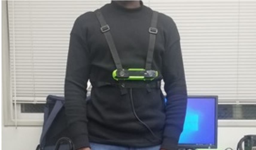
FIGURE 3.8: An image depicting the ZED2 camera being strapped around the chest to capture the front view scene
