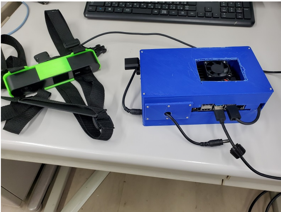
FIGURE 3.9: An image of the 3D printed case holder for the Jetson Nano holder
