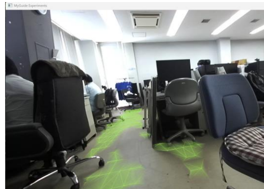
Figure 5 A screenshot of the indoor path selection where the yellow mark safe trails the VIP can walk through.
